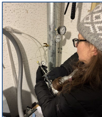
(Left) Air Force environmental contractor monitors SVE system performance.
