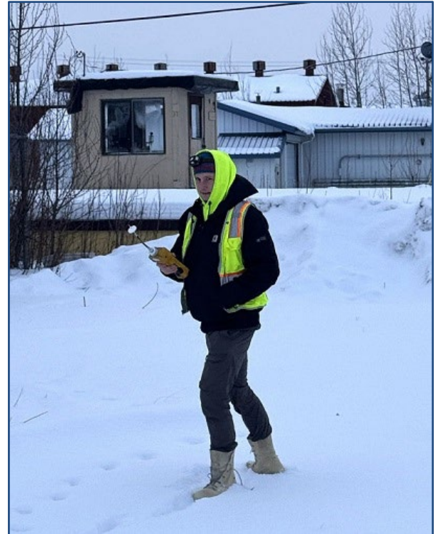
Outdoor air monitoring performed regularly near SVE system exhaust stacks to ensure safe air quality.
